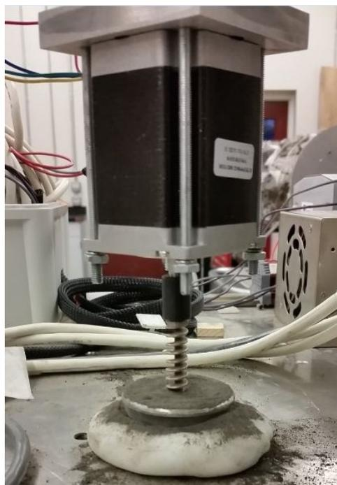
Figure 3: Photo of anchor entering regolith surface during preliminary test trial. Note - In later trials, a larger cup-shaped container replaced the metal hemisphere shown in an attempt to eliminate wall effects.
