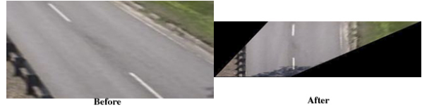
Figure 8: Using of homography to estimate distances
